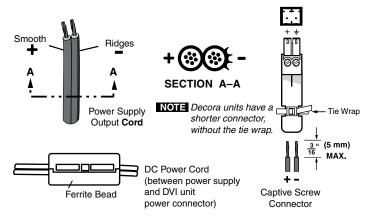
Figure 2-24 — Power connector wiring
